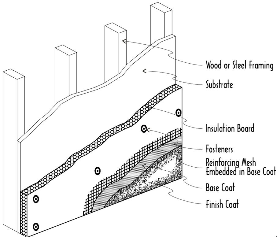
**Fig. 1 STEEL OR WOOD FRAMING**
