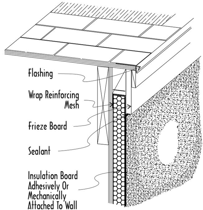
**Fig. 2 NON EIFS SOFFIT**
