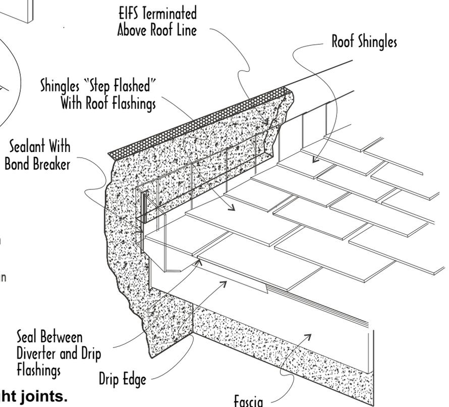
**NOTE: Flashing shall have watertight joints.**
